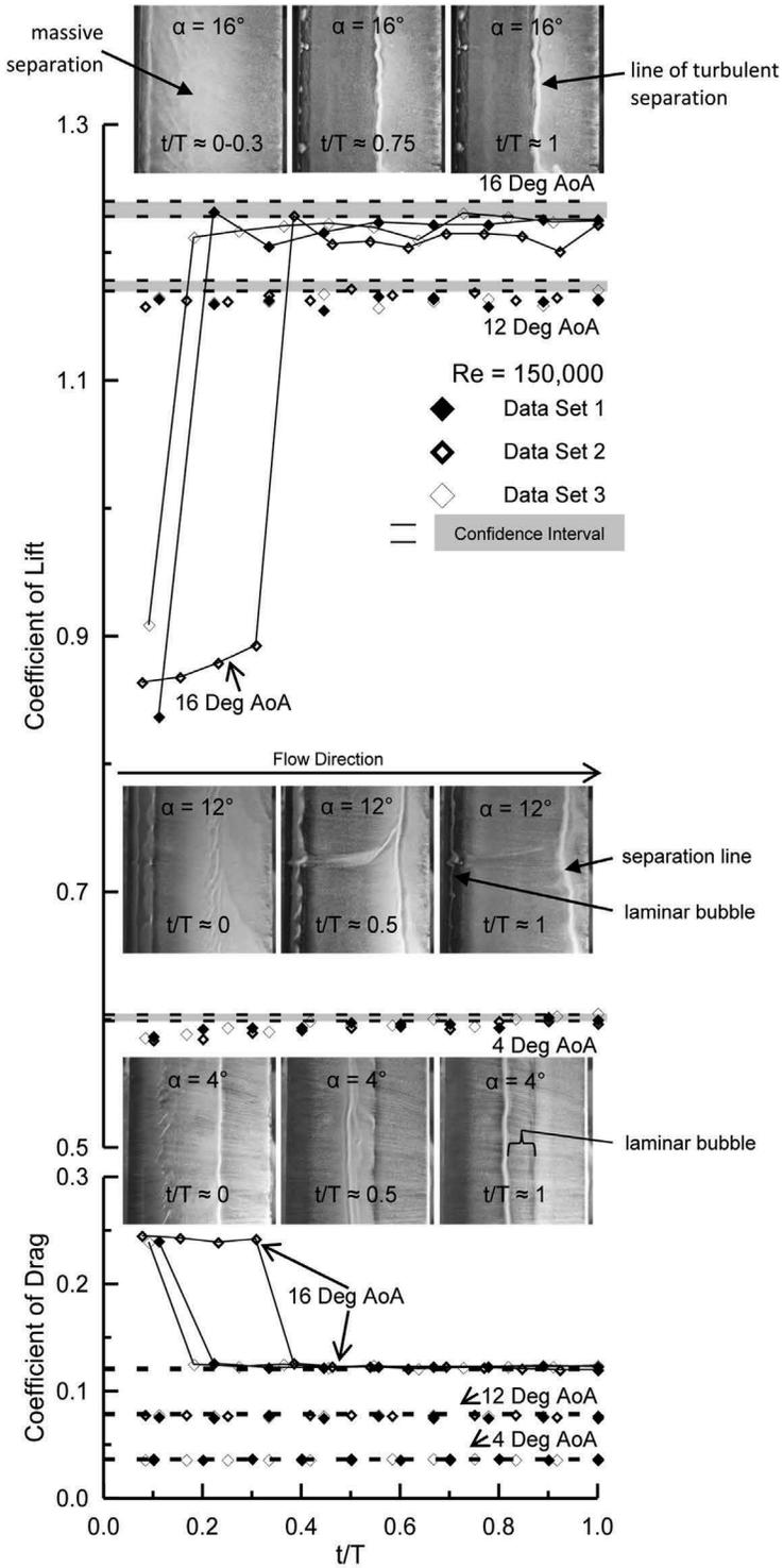
Figure 3. Effect of SFV on temporal evolution of lift and drag coefficient, Re = 150,000.
