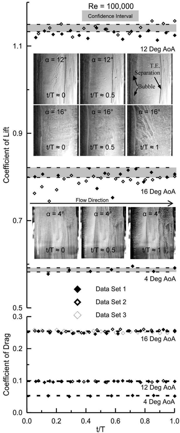
Figure 2. Effect of SFV on temporal evolution of lift and drag coefficient, Re = 100,000.
