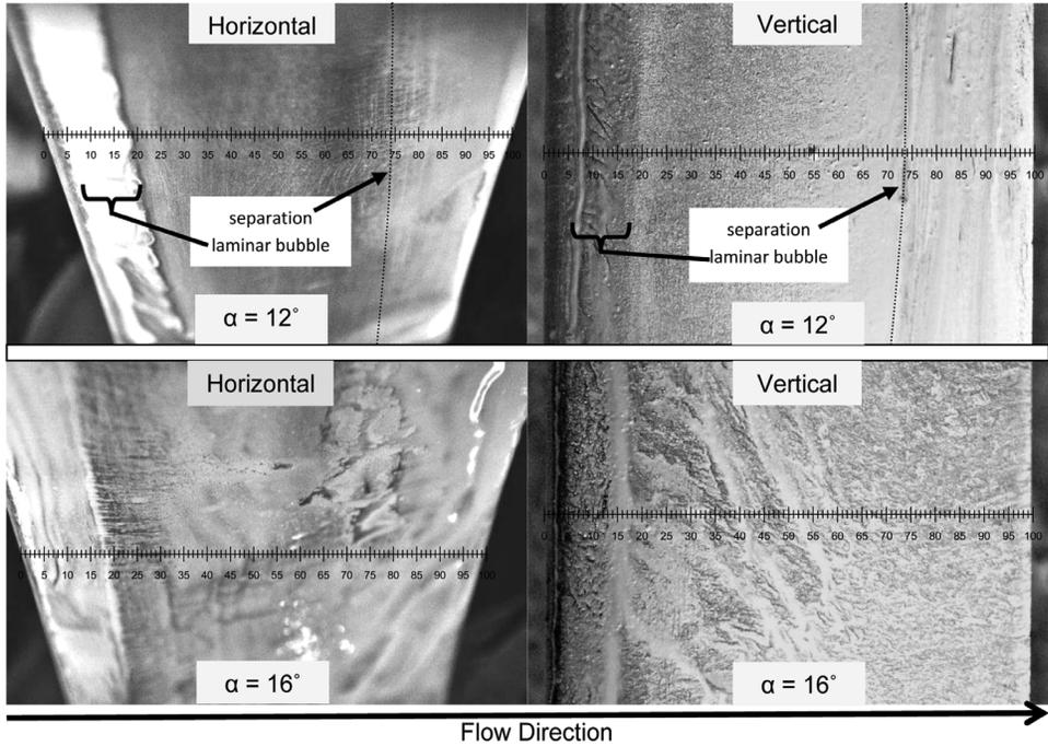
Figure 4. Effect of wing orientation on rendered surface flow patterns. Flow from left to right.
